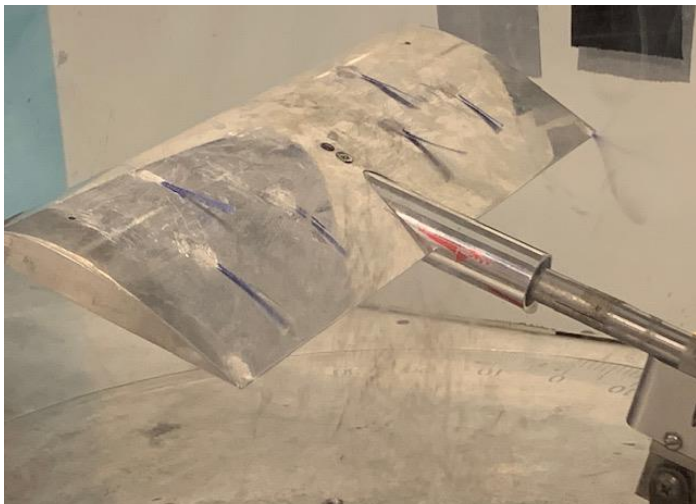
Photo shows the boundary layer beginning to separate from the wing
