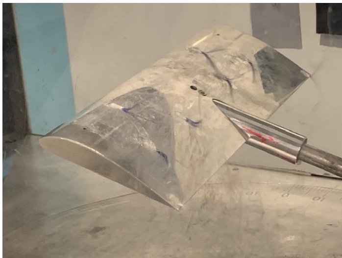
Photo shows the boundary layer beginning to separate from the wing
