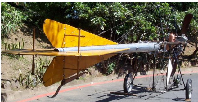
The hollow aluminum & nickel steel empennage.
