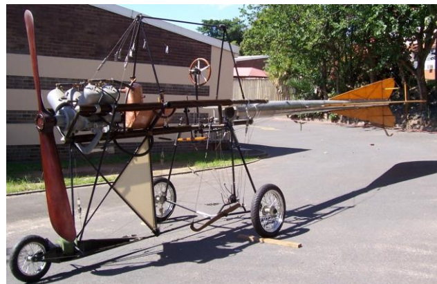
The completed fuse. Note hook break near LH wheel
