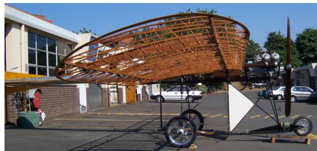
The impressive and time consuming woodwork wings
