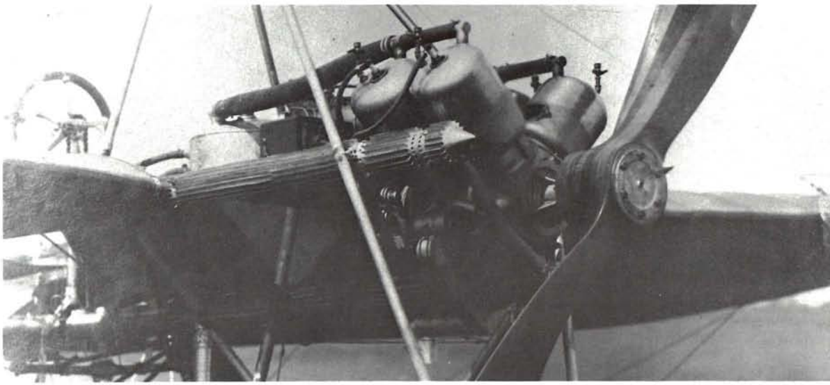
Upper Left: Note the brass steam condenser (tea kettle) just behind the engine. In front of the condenser is the ignition system. Large box was magneto and selective cylinder control, later substituted for blip switch.
