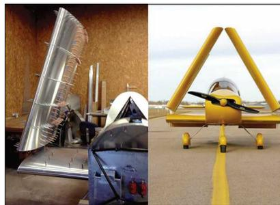
At left is an "Onex" aircraft under construction, and at right is what the finished airplane will look like. Chapter member **Dale Barkley** of Paris, Ill., says he expects to complete the aircraft later this year. The folding wing Onex can be stored in a garage and cruises at 135 mph with fuel economy of 35 mpg.
